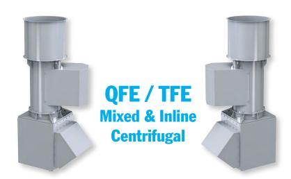
The TFE is an arrangement 9 belt driven inline centrifugal fan that utilizes a high velocity discharge nozzle to achieve a high plume height. The TFE offers a gravity damper at the fan outlet for full positive shut-off when the fan is not in use, which prevents rain from entering the building.
