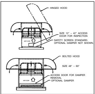
Figure 3. Mounting Roof Ventilator to Curb Cap
