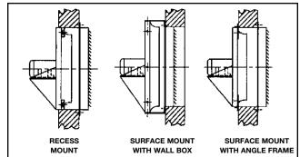
Figure 2. Typical Power Roof Ventilator Installation Arrangements
