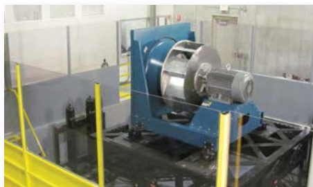
Seismic testing for fans up to 10,000 pounds
