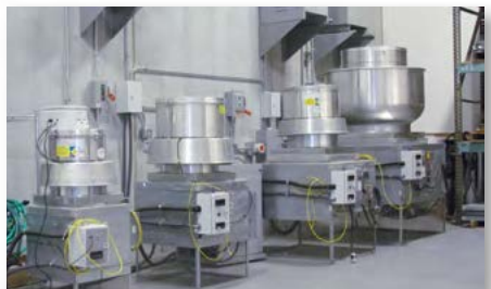
UL 705 safety testing for fans
