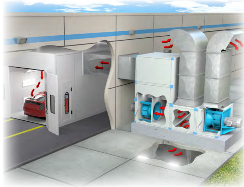
Paint Booth Ventilation
