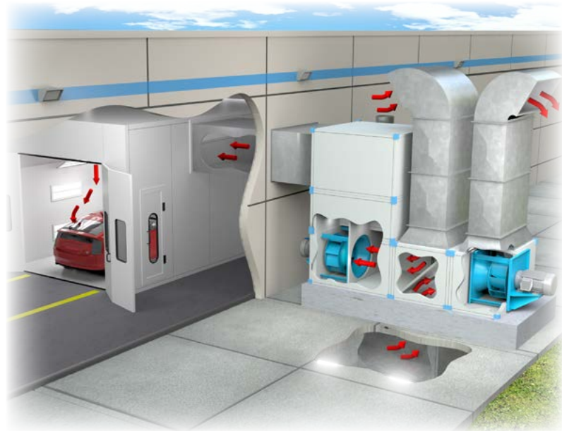
Paint Booth Ventilation
