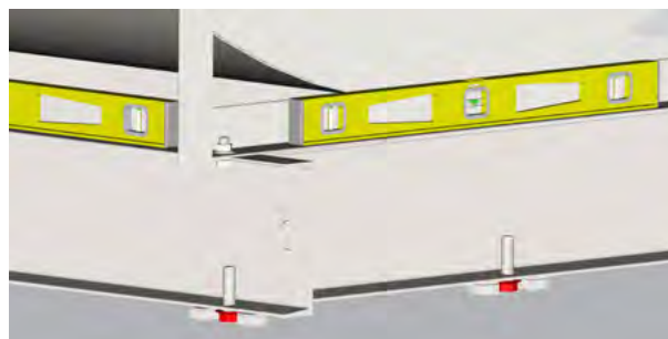
Carefully level the fan on the foundation
