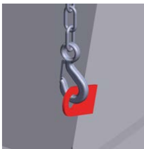
Lifting lugs are provided on most units.
