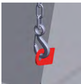
Lifting lugs are provided on most units.
