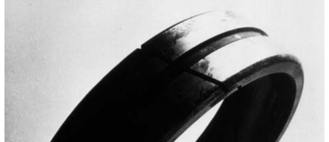
Figure 26. Pits Caused By Electrical Current
