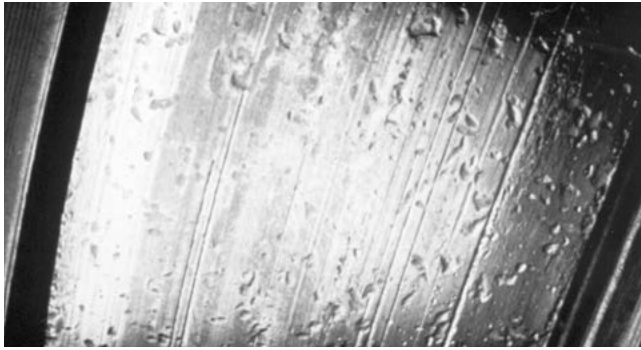
Figure 13. Severe Particle Denting
