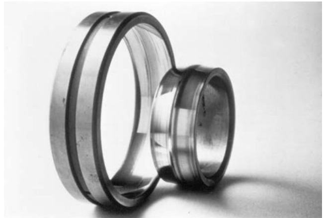
Figure 12. Highly Polished Surfaces Due to Inadequate Lubrication
