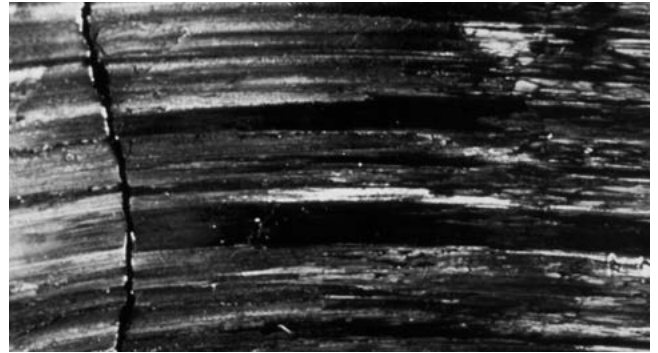
Figure 23. Fretting Corrosion on Bearing Bore
