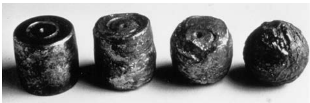
Figure 9. Damaged Spherical Bearing Rollers
