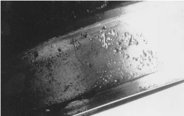
Figure 7. Spalls & Wear Patterns in the Race
