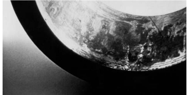
Figure 24. Cracked Inner Race
