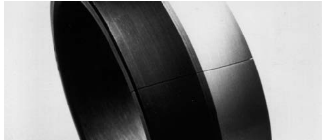
Figure 25. Cracked Outer Race
