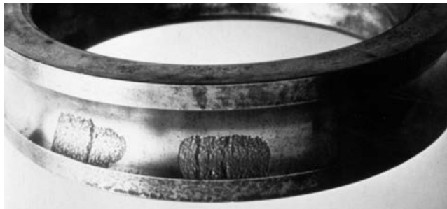
Figure 21. Two Load Zones on the Outer Race
