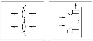
The axial flow fan increases the air velocity through rotational or tangential force, which produces velocity pressure (VP), kinetic energy, with a very small increase in static pressure (SP), potential energy.
