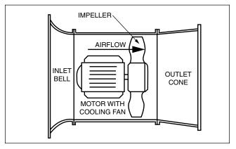
with corrosive chemicals or explosive vapors. They can be mounted in parallel for higher airflows or they can be staged in series to increase their pressure capabilities. Also, as mentioned under the panel fans, using larger hub-to-tip ratio impellers increases the tubeaxial fan's ability to work against pressure for a given speed or conversely enables the fan to work against the same pressure at a lower speed.
