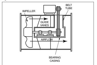
versions. The adjustable pitch versions are limited to clean air applications; however, fans with cast solid impellers can be designed to handle high temperatures and chemical contaminated air. Vaneaxial fans are not recommended for applications containing abrasives, dust, stringy materials or overspray since buildup on the guide vanes will decrease fan performance.
