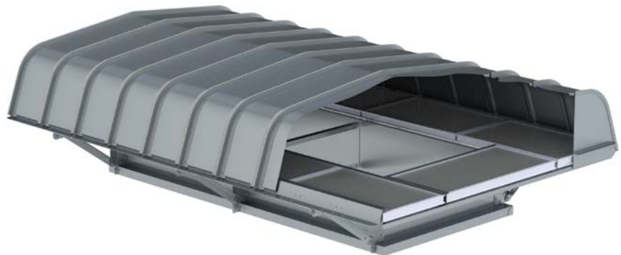
Cutaway view showing the MGI's optional filtered intake construction with 2" aluminum washable filters
