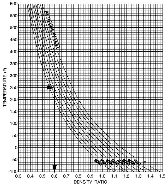
**Example 4:** Select a fan to deliver 8500 CFM at 2½" SP at 5,500 ft elevation at 250°F. From Table 1 the factor for 250°F is 1.34 and from Table 2 the factor for 5,500 ft elevation is 1.22. The overall factor is obtained by multiplying these factors: 1.34 x 1.22 = 1.63. To use a fan manufacturer's performance tables, convert the SP to standard air:
